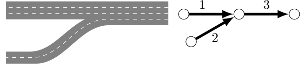
Fig. 5. Sketch of a merging junction consisting of three links.
