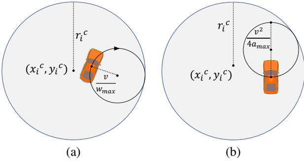
Fig. 2: (a) An autonomous vehicle executing an evasive maneuver of  $[0, -\omega_{max}]$ . In this figure,  $h_i^t(x, y, v, \theta) = 0$ . (b) An autonomous vehicle executing an evasive maneuver of  $[-a_{max}, 0]$ . In this figure,  $h_i^b(x, y, v, \theta) = 0$  as well.
