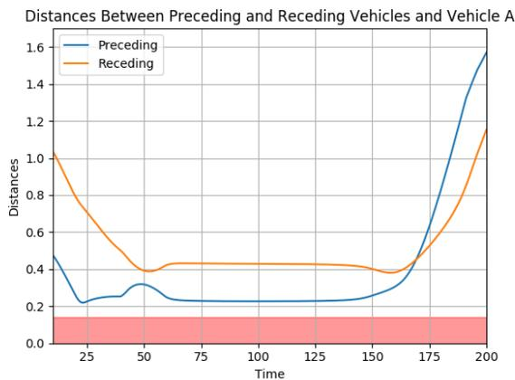
Fig. 4: Distances between vehicle  $A$  and the preceding and receding vehicles are depicted. The distances between the vehicles never violate the collision avoidance safety specification, shown as the shaded region.
