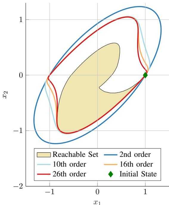
Fig. 1: Simulated system response of (18). When starting from  $x_0 = [1, 0]^T$ , the system can only reach the region shown in light yellow, which was computed via simulation. The dark blue, light blue, orange and red regions represent invariant sets calculated using quadratic, 10<sup>th</sup>-order, 16<sup>th</sup>-order and 26<sup>th</sup>-order meta-Lyapunov functions, respectively. The invariance of these regions is shown by (19).
