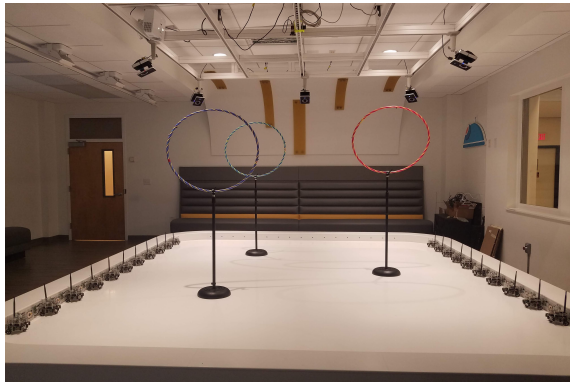
(a) The hoops are mounted on adjustable stands and are tracked via Vicon markers.
