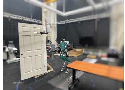
(c) Hardware set-up with a Digit walking robot and a quadcopter
