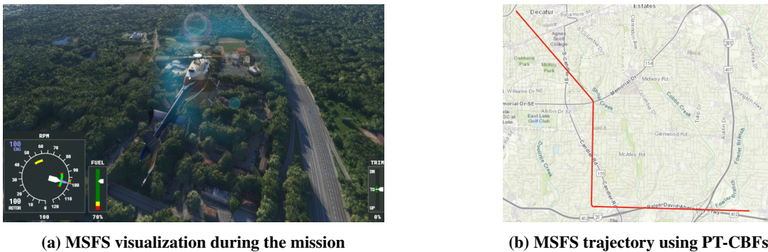
Fig. 5 Microsoft Flight Simulator example. The system tracks three ordered waypoints ( 33.7157^\circ N, 84.2821^\circ W ), ( 33.7472^\circ N, 84.2821^\circ W ), and ( 33.7759^\circ N, 84.3107^\circ W ), but it is not allowed in their proximity before T_{safe} expires.
