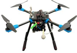
**Fig. 3.** The Holybro x500v2 quadrotor used for hardware experiments. It is fitted with tracking markers, a radio receiver, and an on-board Raspberry Pi with ROS2 for control computations. The quadrotor weighs 1.69 kg and is 0.5 m diagonally.
