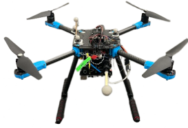
Fig. 8. The Holybro X500 V2 quadrotor used for hardware experiments. It is fitted with tracking markers, a radio receiver, and an on-board Raspberry Pi with ROS2 for control computations. The quadrotor weighs 2.1 kg, measures 0.6 m diagonally, and 0.25 m vertically.
