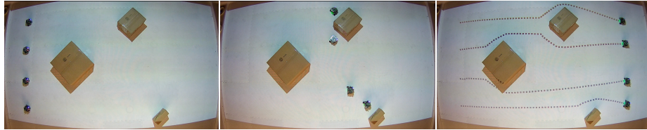
Fig. 4. Four GTernal robots successfully navigating to their goal positions without colliding with unknown obstacles in the arena utilizing their onboard collision avoidance algorithm.
