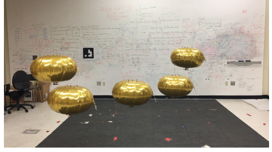
Fig. 2: Flight trajectory of the GT-MAB during the experiment in 3D space. The blimp on the left is the starting point of the sequence and the blimp on the right is the ending point of the sequence.
