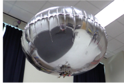
Fig. 5. The GT-MAB research blimp used to collect the pose-labeled image dataset.
