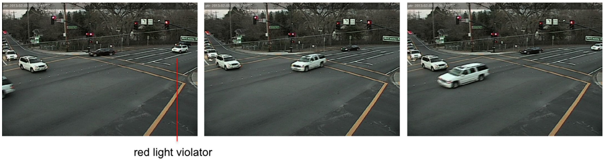
Fig. 12. A near crash between a red light violator and a conflicting entry. (For interpretation of the references to color in this figure legend, the reader is referred to the web version of this article.)
