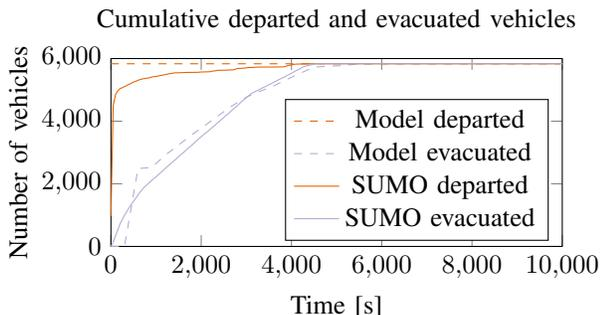
Fig. 4. Cumulative departures and number of evacuated vehicles when all the vehicles are instructed to depart at once. The cumulative curve of evacuated vehicles based on the model reflects the curve of evacuated vehicles observed in the microscopic traffic simulator.
