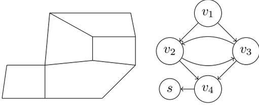
Fig. 1. Example of how different sectors in a region targeted for evacuation can be mapped to the corresponding graph representation.
