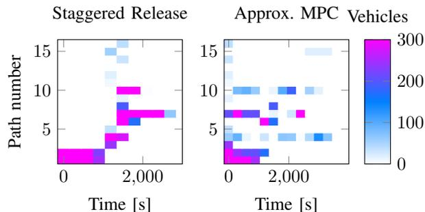
Fig. 7. The number of vehicles released at each time for each path with a staggered release approach and an approximate MPC approach.
