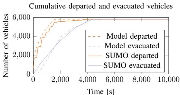
Fig. 5. Cumulative departures and number of evacuated vehicles with a fixed departure rate of 200 vehicles per path every fifth minute. The cumulative curve of evacuated vehicles based on the model reflects the curve of evacuated vehicles observed in the microscopic traffic simulator.
