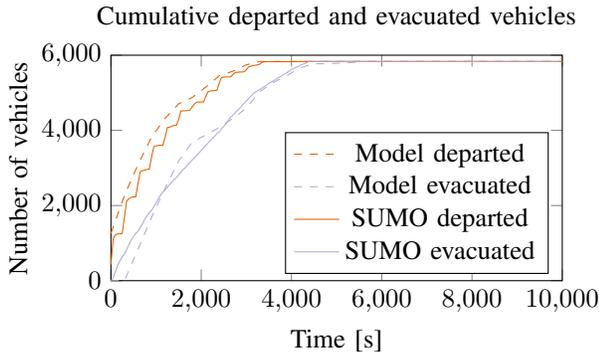
Fig. 9. Cumulative departures and number of evacuated vehicles when the vehicles are released according to the approximate MPC strategy.
