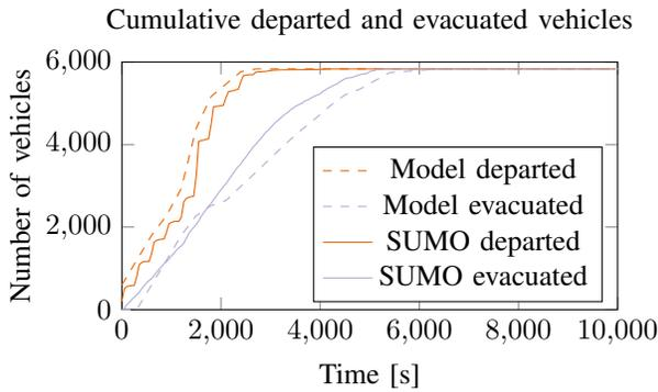
Fig. 8. Cumulative departures and number of evacuated vehicles with a staggered release approach.
