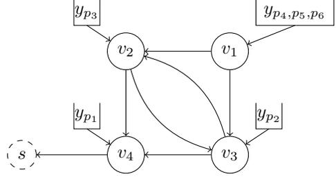
Fig. 2. Example of a city with four sectors, where each of the sector has one or several path dependent input buffers with vehicles that should be released. Once the vehicles are released, they will travel to the safe sector, node  $s$ . In this example, the set of paths is  $\mathcal{P} = \{p_1 = (v_4, s), p_2 = (v_3, v_4, s), p_3 = (v_2, v_4, s), p_4 = (v_1, v_2, v_4, s), p_5 = (v_1, v_3, v_4, s), p_6 = (v_1, v_2, v_3, v_2, v_4, s)\}$ .
